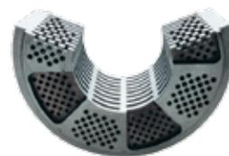
Variable Resistance Trim (VRT\*), consists of a brazed stack of drilled plates which efficiently channel the flow through multiple turns in a tortuous path configuration. The design is primarily used in high-pressure drop liquid applications. VRT is typically packaged within standard Masoneilan globe and angle valve bodies.
